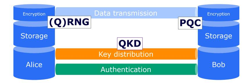
QKD for distributing secure symmetric keys Data transmission is still a classical process A classical authenticated channel needed -> ID Systems All other parts needed to be classically secured -> PQC, crypto agility
