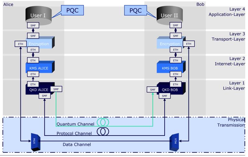
Legend: SMF – Singlemode Fiber ETH – Ethernet Port KMS – Key Management System (DE)MUX – (De)Multiplexer ←→ - Physical Connection
